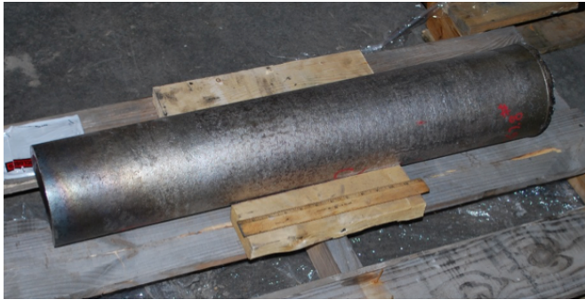
Figure 8.11: As cast 300-lb VIM/VAR heat of QT-Co
