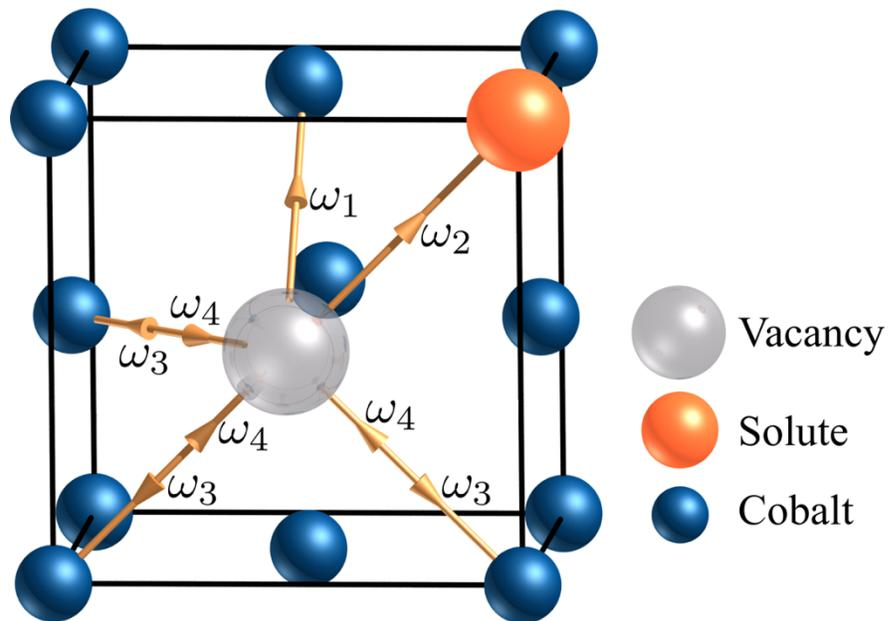
**Caption:** Vacancy jumps in fcc cobalt near an impurity. The orange ball is the impurity and empty gray ball indicates the vacancy.  $\omega_0$ : vacancy-host exchange rate.  $\omega_1$ : rotation rate of impurity-vacancy.  $\omega_2$ : impurity-vacancy exchange rate.  $\omega_3$ : dissociation rate of impurity-vacancy pair.  $\omega_4$ : association rate of impurity-vacancy pair.
