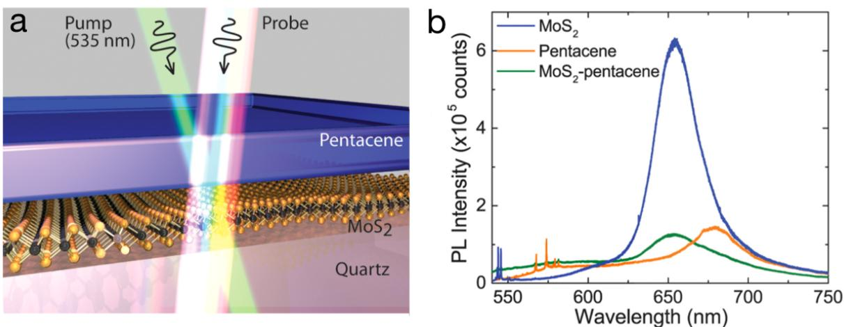
**Caption:** (a) Schematic depiction of the vertical pentacene-monolayer MoS<sub>2</sub> p-n heterojunction being probed by transient absorption spectroscopy. (b) Photoluminescence spectroscopy of the pentacene-MoS<sub>2</sub> heterojunction and its constituent materials, showing quenched MoS<sub>2</sub> photoluminescence in the type-II heterojunction.
