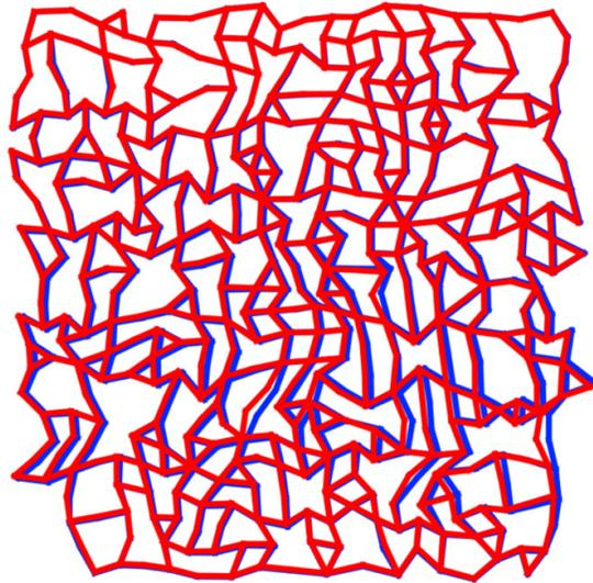
**Caption:** A compressed 500-node experimental network with comparison to simulation. Image compares the experimental configuration with that predicted from simulation at a strain in the vertical direction of 0.04. In red is shown a rendering of the experimental configuration and in blue is shown the simulated configuration at the same strain.
