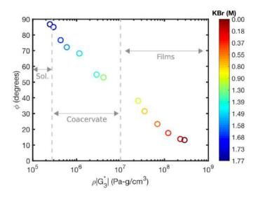
Figure 4.3: The mechanical response of a polyelectrolyte complex composed of polystyrene sulfonate and poly(diallyldimethyl chloride) (PSS:PDADMAC) as a function of salt concentration. The quartz crystal microbalance was used to quantify the continuum of mechanical properties assumed by PSS:PDADMAC, elucidating the transition from films to coacervate to a single phase solution.
