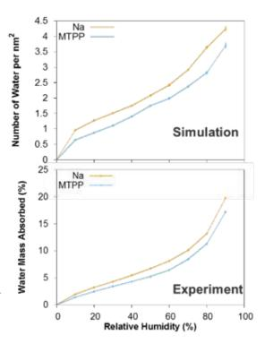
Figure 5.5: The absorbed water mass and surface tension of CNCs with different surface modifications.
