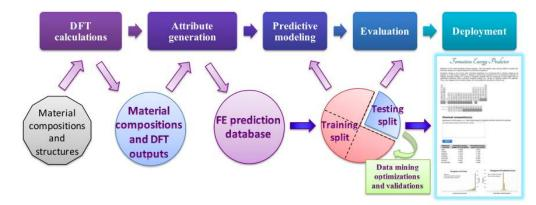
Figure 12.2: The design of the data mining workflow used to build formation energy prediction models. DFT calculations on hundreds of thousands of compounds have been done and stored in OQMD. Only composition information was used to derive additional attributes and build ensemble predictive models. The most accurate models were deployed in the online formation energy predictor tool.
