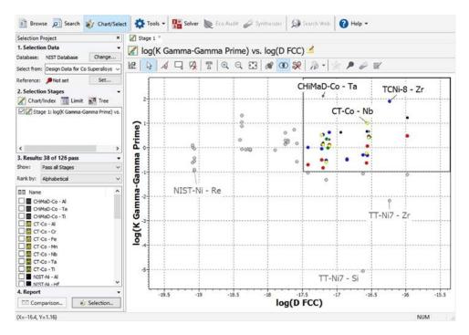
Figure 6.8: A data plot generated by CES Selector can save users time by making data of interest more prominent and easier to find. Shown here are the results of a one-step graphical box selection of Cobalt phase data gathered by ChiMaD PIs
