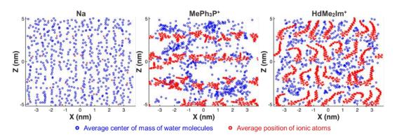
Figure 5.6: Predicted distribution and orientation of water molecules around the ions on the surface of modified CNCs.
