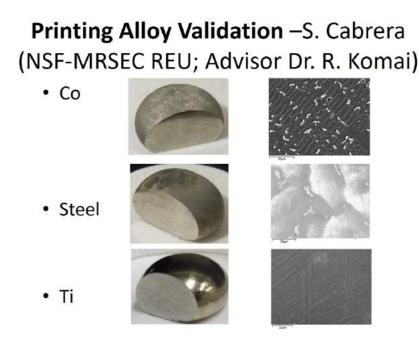
Figure 6.21: Compositions designed from MSE 390 regarding a 3D printed Cobalt, Steel, and Titanium alloy were prototyped by CHiMaD REU student Samuel Cabrera (UCI). Alloy prototypes were then heat treated and examined for 3D printing feasibility.
