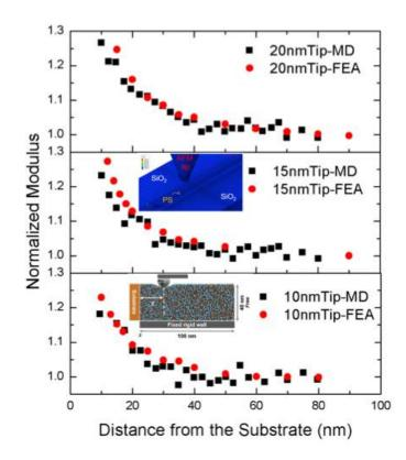
Figure 5.8: Effects of AFM tip radius via MD and FEA confirm impact of substrate stress field interaction
