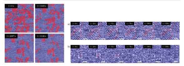
Figure 3.6: Left: AFM images of the *PS-b-PMMA* during in situ thermal annealing. The area fraction of the defective domains were tracked over time to analyze kinetic data. Right: A time sequence of *PS-b-PMMA* on unpatterned substrate during in situ thermal annealing at 210°C shows repeated disconnections and reconnections of strained junctions; in contrast, assembly on chemically patterned substrate shows the irreversible conversion of a stitched domain to aligned lamella.
