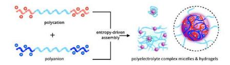
Figure 21.5: Illustration of polyelectrolyte complex (PEC) assembly process from tailorable polycations and polyanions. The effects of new polymer platforms with modular ionic character, molecular architecture, and chemical moieties on resultant mechanical, rheological, and responsive PEC properties will be pursued.
