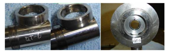
Figure 6.16: QT-Co alloy bushings after wear testing, showing low wear on both the bushing and the Cr-plated pin, indicating successful testing
