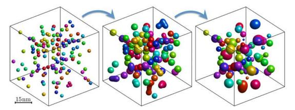
Figure 11.2: Growth of  $\gamma'$  precipitates in a  $\gamma$  matrix at times 1h10min (left), 3h32min (middle), and 19h00min (right) of aging time
