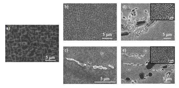
Figure 6.3: Secondary electron SEM micrographs of Co-Ni-Al-W-Ti-Ta-Cr alloys aged at 900°C for 168h with: a) 0 at% Cr, b) 4 at% Cr, c) 8 at% Cr, d) 12 at% Cr, d) 16 at% Cr.
