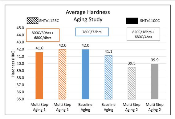
Figure 6.15: Aging study performed on QT-Co at various solution heat treatment times and aging treatments, which show similar hardness values for both the baseline aging treatment and the multi-step aging treatment 1 (HRC 41.5-42
