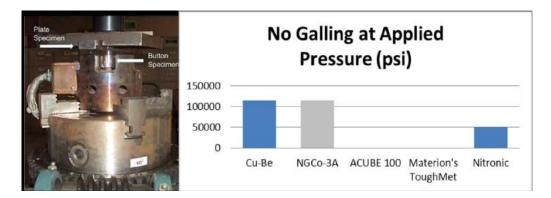
Figure 6.18: Photo of the galling resistance test setup (left), and *Northrop Grumman*-collected ASTM G98 galling test data (right), of QT-Co which shows similar results to Cu-Be in evaluation (i.e, no galling up through all tested stresses). ACUBE 100 and Toughmet (shown in this plot) were evaluated by *Northrop Grumman* in this initial test plan but were not selected for Galling evaluation
