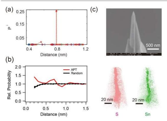
Figure 2.2: (a) Probabilities of the occurrence of Ag - Ag configurations at 300K from DFT calculations. (b) Ag - Ag radial distribution function from APT reconstruction compared with that of Ag atoms randomly substituted for Bi and Pb atoms. (c) SEM image of a sharpened tip from a Ag - SnS - Ag sandwich structure and the distribution of S and Sn in the APT reconstruction.
