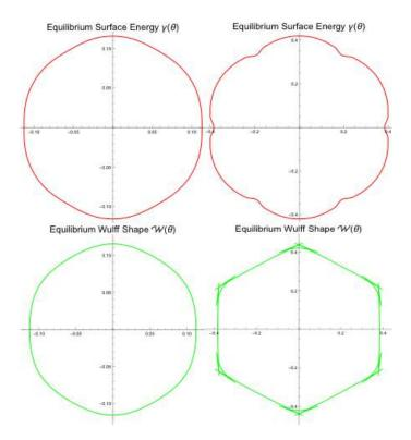
Figure 21.2: Equilibrium Surface energy and Wulff Shape in polar coordinates. System temperature decreases from left to right, with the top row showing the surface energy while the bottom row shows the Wulff shape construction. Note the emerging cusps (rounded) in the surface energy and the accompanying emergence of ears in the Wulff construction.
