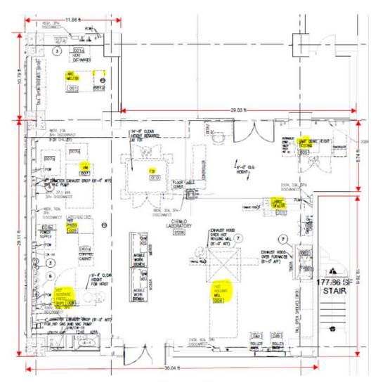
Figure 13.1: Plan of the CHiMaD Metals Processing Facility, designed with current and future equipment in mind.
