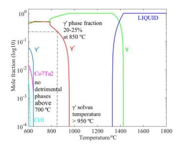
Figure 6.7: Step diagram of the designed Co-based superalloy
