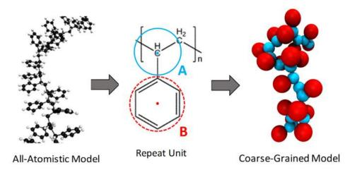
Figure 21.4: The atomistically informed coarse-grained model of polystyrene, showing the mapping from (left) all-atomistic (AA) model to (right) coarse-grained (CG) model. (Middle) For each repeat unit, backbone type "A" CG bead is centered on the alkyl carbon bonded to phenyl ring. Side chain type "B" CG bead is located at the center mass of the phenyl ring.
