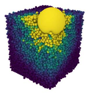
Figure 9.1: A snapshot from the new simulation code, showing a spherical impactor indenting a three-dimensional granular medium, with colors indicating the magnitude of the contact forces between neighboring particles (the image shows a corner cut through the 3d granular medium to better highlight the stress penetration, the simulated material extends beyond the corner; colors: yellow to blue = high to low contact force magnitudes)
