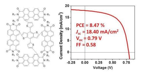
Figure 7.1: Molecular structures of  $\alpha$ TPB and J-V curves of binary solar cells (PTB7-Th: $\alpha$ TPB).
