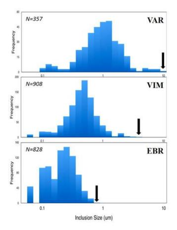
Figure 6.12: Process Optimization for Inclusion Refinement: Comparison of histograms of inclusion sizes ( $\mu m$ ) produced in NiTi tubes in vacuum arc remelting (VAR), vacuum induction melting (VIM), and electron beam refining (EBR). EBR material indicates a smaller inclusion size, which indicates fatigue life may be improved when NiTi tubes are produced by this process.
