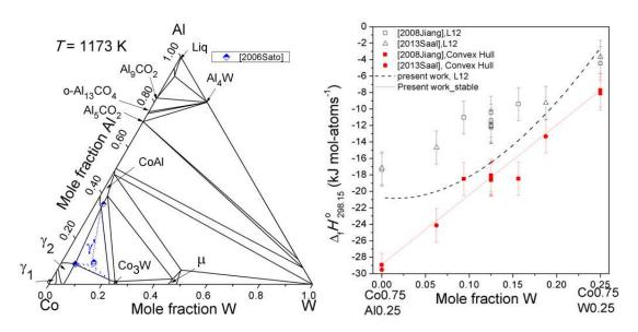
Figure 21.3: From left to right: (A) Calculated isothermal section at  $1173^{\circ}K$  with calculated metastable  $\gamma'$  phase equilibria superimposed. (B) Calculated enthalpy of formation of the  $\gamma'L1_2$  phase and enthalpy of formation for the stable status compared with DFT results from literature DFT error bars were assessed as 2kJ.
