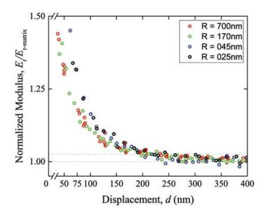
Figure 5.9: Interphase length scale in PS-silica system with substrate stress field interaction removed
