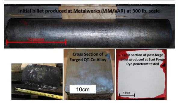
Figure 6.14: QT-Co alloy prior to forging (upper), post forging (lower left); cross-sectioned (middle); and (right) dye penetrant tested to ensure crack-free core
