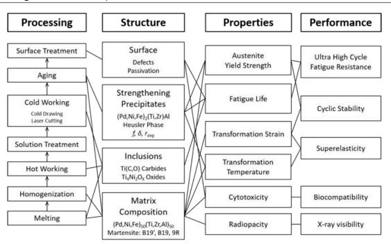
Figure 6.2: Systems design chart of High-Performance Shape Memory Alloys
