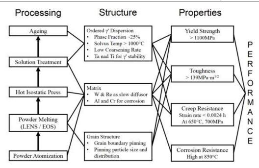
Figure 6.6: System design chart showing the process-structure-property relation for a Co-based superalloy designed for additive manufacturing
