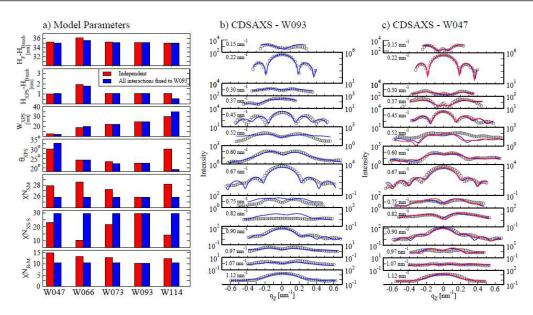
Figure 3.3: Theory and simulation based analysis of X-ray scattering experiments. A single set of material parameters (a) were used to successfully fit the scattering profiles from samples with different template geometries (b) (c). The fine-tuned parameters can then be used for predictive modeling.
