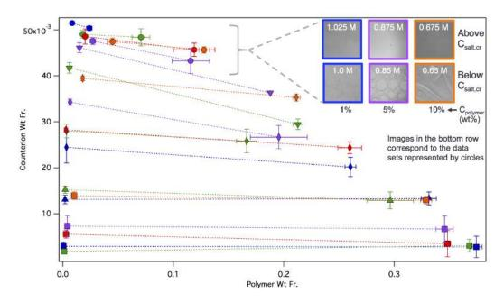
Figure 4.4: Counterions-polymer phase diagram for associative phase separation between polylysine and polyglutamic acis at various polymer concentrations and added salt concentrations
