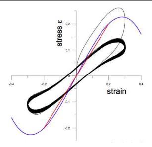
Figure 6.13: Dynamic stress-strain curve of cyclic loading
