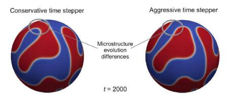
Figure 11.1: Snapshot of the microstructure evolution for spinodal decomposition on the surface of a sphere. The figure illustrates differences obtained with different time steppers at a snapshot in time: the left figure is generated using a conservative time stepper, and the right figure an aggressive time stepper.
