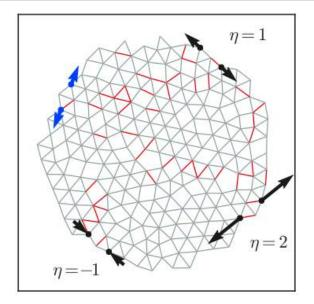
Figure 9.2: Network with 200 nodes and 502 bonds with an average coordination number of 5.0. The network was tuned to show responses at three target sites (shown by the black arrows) with responses of  $\eta = 1, 2and - 1$  where  $\eta$  is the ratio of the output to the input strain. All three targets are controlled by a single pair of source nodes shown by the blue arrows.
