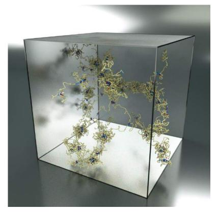
Figure 21.1: Snapshot from MD simulation of triblock copolyelectrolytes assembly (40-200-40 ABA triblock at 0.36wt% polymer concentration). Charged end-blocks (blue and red) form polyelectrolyte complex cores, while midblocks (yellow) make up a percolating structure, resulting in gel-like material.
