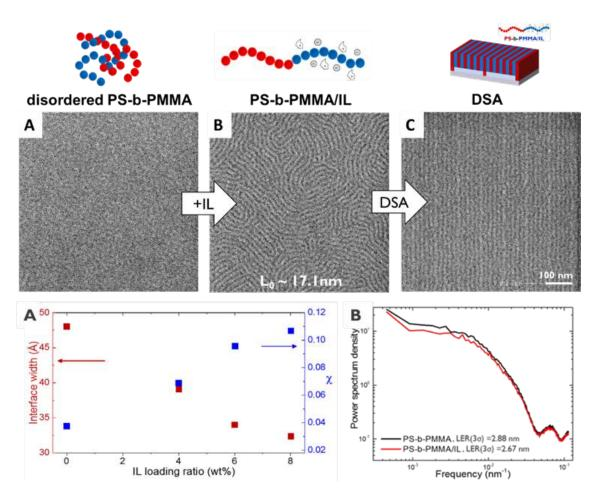
Figure 3.4: Top: (A-C)Addition of ionic liquid facilitates the phase separation of PS-b-PMMA and DSA of 8.5 nm half-pitch lines were demonstrated, Bottom: (A-B) Reflectivity experiments in collaboration with NIST showed that ionic liquid increased the Flory-Huggins parameter between the polymer blocks and reduced the interfacial width.
