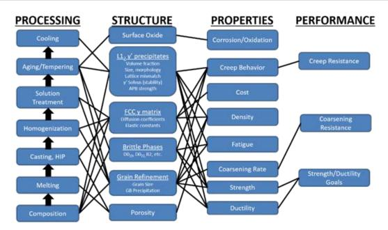
Figure 6.1: Systems design chart of Cobalt Superalloys
