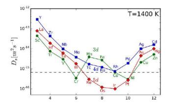
Figure 6.10: Relative Diffusivity of solutes in a Co-matrix at  $T = 1400^{\circ}K$
