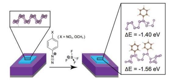
Figure 2.1: Depiction of the reaction scheme of benzene-diazonium tetrafluoroborate derivatives with 2D black phosphorus (blue) on a  $SiO_2$  (purple) on Si (gray) substrate. The calculated lattice distortions resulting from adsorption of the aryl groups, and their respective adsorption energies, are shown on the right.
