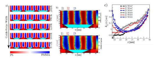
Figure 3.1: 3D Characterization of DSA using CDSAXS. (a) Average cross-sections for samples with different template critical dimensions showing shape variations through the film thickness. (b) Positional fluctuations of the interface with regard to its location on the template. (c) Fluctuation profile in the thickness direction showing increased fluctuations at the top surface.
