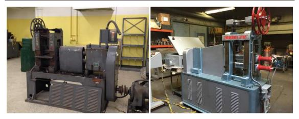
Figure 13.3: (*Left*) Fenn 2/4 Hi Rolling Mill shown before refurbishing. (*Right*) A representation of how Fenn 2/4 Hi Rolling Mill is expected to look after refurbishing
