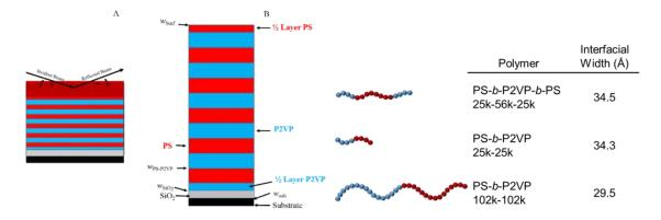
Figure 3.5: (Left) Soft X-ray reflectivity experimental setup. (Right) Interfacial widths for polymers with different architectures and molecular weights.
