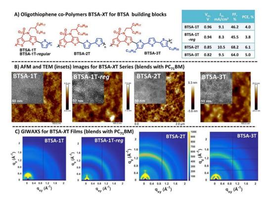
Figure 7.3: BTSA-XT co-polymers: A) Chemical structures and summary of BHJ OPV cell performance; B) AFM (height) and TEM images; C) GIWAXS diffraction images. All films were spin-coated using 5 mg/mL (polymer concentration) solution in CF:DCB (9:1) solvent mixture with 2% of DIO (1,8-diiodooctane) processing additive. Polymer:fullerene ( $PC_{71}BM$ ) = 1:2 weight ratio was used.
