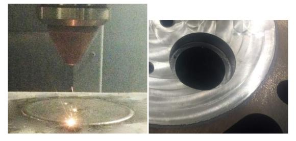
Figure 8.1: From Left to Right: (A) Laser deposition repair process (B) Completed Laser deposition repair
