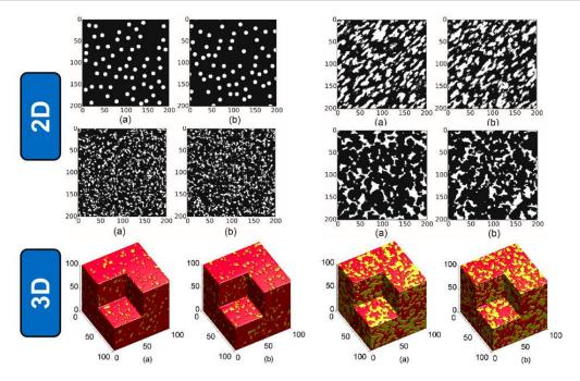
Figure 12.7: Reconstruction through Supervised Learning: Reconstructed images in (b) are statistically equivalent to the original images in (a). The method is shown to be effective for a broad range of microstructures.
