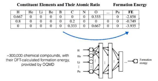
Figure 12.5: Schematic for deep learning system. The training algorithm learns the relationship between the input elemental fractions and output formation energy via multiple hidden layers of neurons, without any additional hand-engineered attributes.
