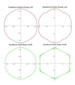
Figure 11.4: Equilibrium surface energy and Wulff Shape in polar coordinates. System temperature decreases from left to right, with the top row showing the surface energy while the bottom row shows the Wulff shape construction. Note the emerging cusps (rounded) in the surface energy and the accompanying emergence of ears in the Wulff construction.
