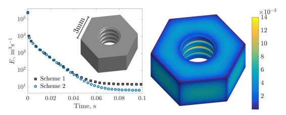
Figure 11.3: Energy functional of the two schemes during simulated heat transfer in an industrial component (left), relative deviation of the determined solution and the exact boundary condition at the component interface at t=15ms
