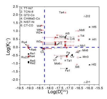
Figure 6.5: Map of elemental partition coefficient between  $\gamma$  and  $\gamma'$  and the diffusivity in matrix at 900°C. Red denotes Co-databases.
