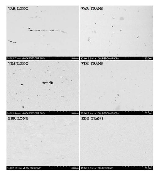
Figure 6.11: Representative backscatter electron micrograph of inclusion microstructure of NiTi tubes produced by vacuum arc remelting (VAR), vacuum induction melting (VIM), and electron beam refining (EBR).
