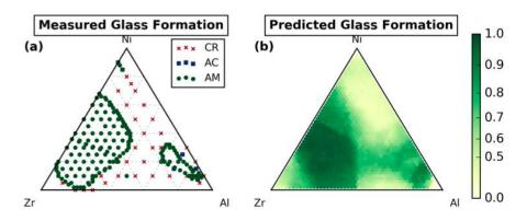
Figure 12.3: (Left) Experimentally-measured regions of glass-forming ability in the Al-Ni-Zr ternary system. (Right) Predicted glass-forming ability by a machine learning model that was trained without any data from the diagram present on the left
