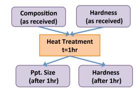
Heat treatment (ex. B -> B') does not transform the composition, but it does transform the hardness and ppt. size.
