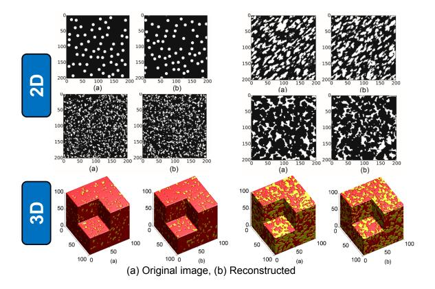
*Caption:* Reconstruction through Supervised Learning: Reconstructed images in (b) are statistically equivalent to the original images in (a). The method is shown to be effective for a broad range of microstructures.
