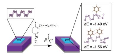
**Caption:** Depiction of the reaction scheme of benzene-diazonium tetrafluoroborate derivatives with 2D black phosphorus (blue) on a SiO<sub>2</sub> (purple) on Si (gray) substrate. The calculated lattice distortions resulting from adsorption of the aryl groups, and their respective adsorption energies, are shown on the right.
