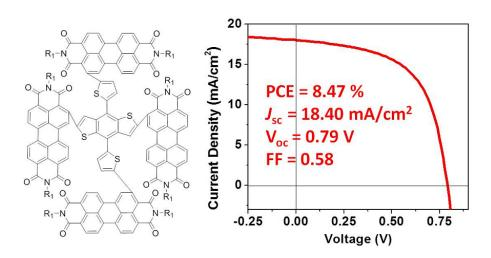
**Caption:** Molecular structures of  $\alpha TPB$  and J-V curves of binary solar cells (PTB7-Th: $\alpha$  TPB).
