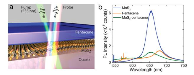
**Caption:** (a) Schematic depiction of the vertical pentacene-monolayer  $MoS_2$  p-n heterojunction being probed by transient absorption spectroscopy. (b) Photoluminescence spectroscopy of the pentacene- $MoS_2$  heterojunction and its constituent materials, showing quenched  $MoS_2$  photoluminescence in the type-II heterojunction.
