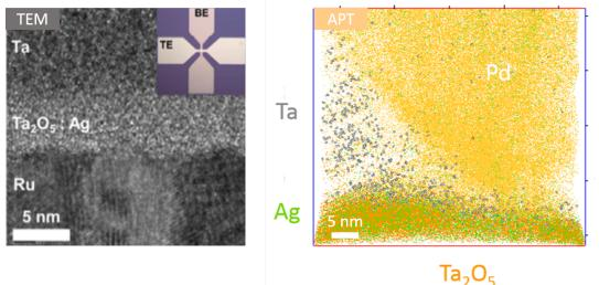
**Caption:** The left panel shows cross-sectional high resolution TEM image of a memristor device with a top view image inset. The right shows an APT reconstruction ( $50x45 \text{ nm}^2$ ) of a specimen targeting the edge of a memristor crossbar device, with yellow dots for Pd, gray dots for Ta, orange dots for Ta<sub>2</sub>O<sub>5</sub> and green dots for Ag. Pd was deposited to protect Ta from oxidation.
