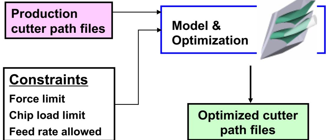
Machining process optimization reduces cycle time and increases cutter survival rate
