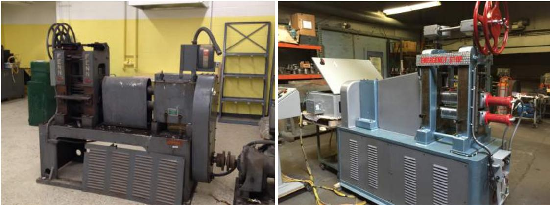
Figure 13.3: (Left) Fenn 2/4 Hi Rolling Mill shown before refurbishing. (Right) A representation of how Fenn 2/4 Hi Rolling Mill is expected to look after refurbishing
