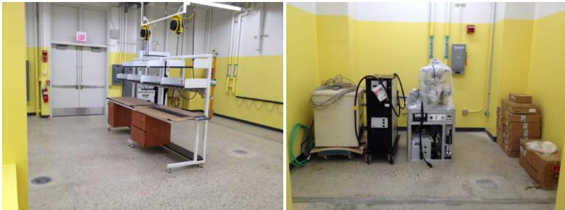
Figure 13.2: (left) CHiMaD Materials Processing Facility as construction was completed, (Right) The first equipment to be moved in was the Buehler AM/0.5 Arc Melter
