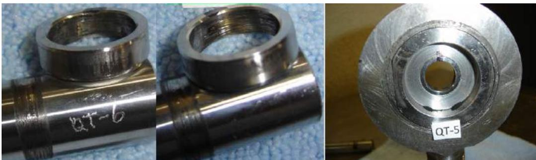
Figure 6.16: QT-Co alloy bushings after wear testing, showing low wear on both the bushing and the Cr-plated pin, indicating successful testing
