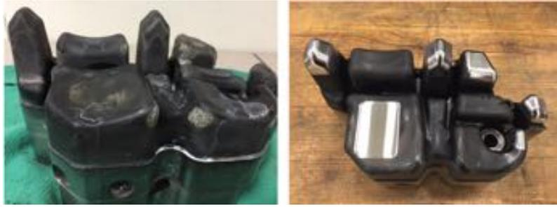
Figure 8.8: (Left) Die Condition prior to repair; (Right) Repaired die.
