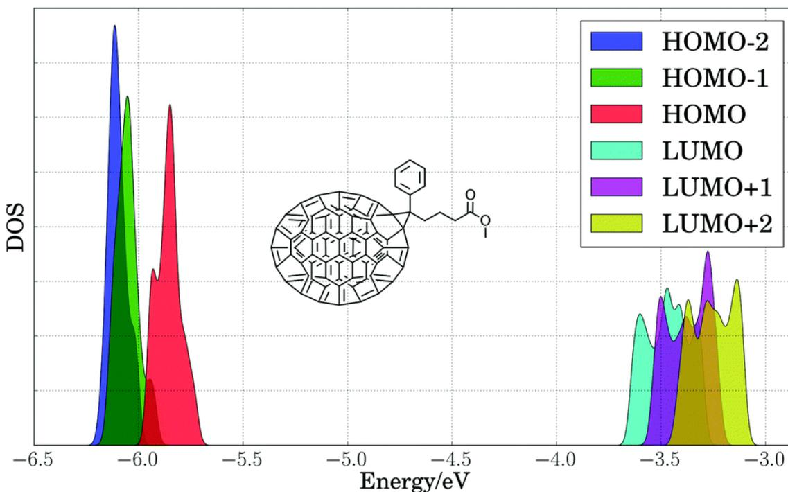
**Caption:** Density of states (DOS) of calculated B3LYP HOMO-2, HOMO-1, HOMO, LUMO, LUMO+1, and LUMO+2 energy levels (eV) for 80 PC71BM configurations, with each energy level marked by color. A Gaussian broadening of 0.02 eV was applied to computed energy levels.
