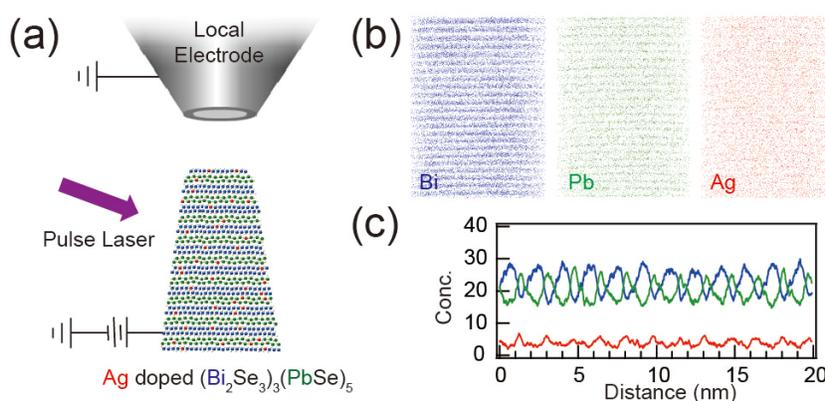
**Caption:** (a) Schematic of atom probe tomography measurement. (b) Reconstruction showing the distribution of Bi, Pb and Ag. The layered structure is resolved. (c) 1D concentration profiles of Bi, Pb and Ag.
