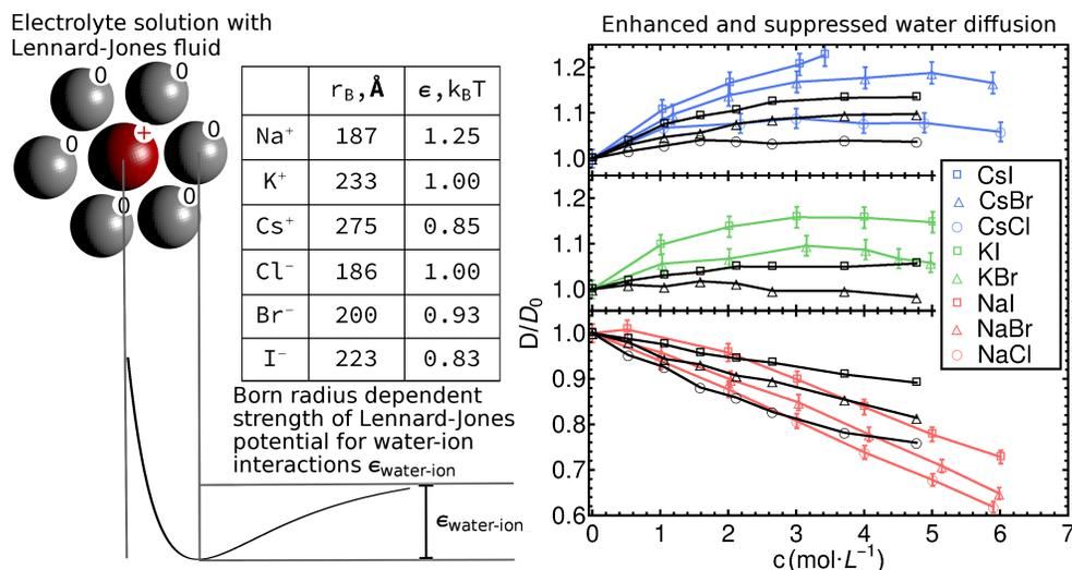
**Caption:** Left: Outline of modeling approach. The strength of Lennard Jones interaction between ion and solvent bead is adjusted according to experimental values of Born radius. The strength for several ions are summarized in the table. Right: Comparison of calculated and experimental diffusion coefficients for several salt solutions. Both enhanced and suppressed diffusion is captured.
