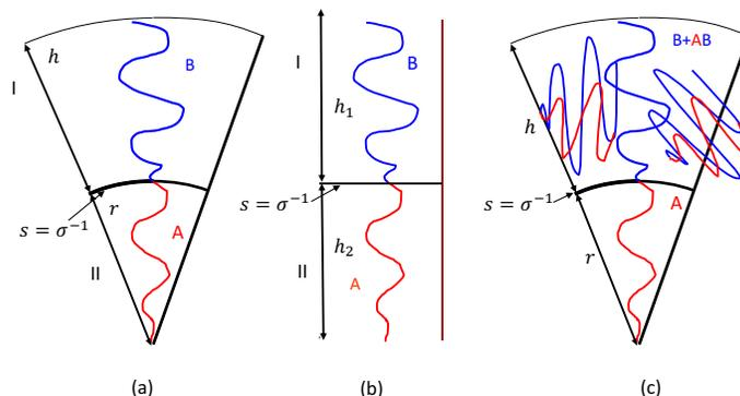
**Caption:** Schematic of the different morphologies in charged (B) and -neutral (A) copolymers: (a) cylindrical or spherical morphologies with an A core; (b) lamellar morphologies; (c) cylindrical or spherical morphologies with the core of pure A component, and the corona composed of a mixture of B+AB components.
