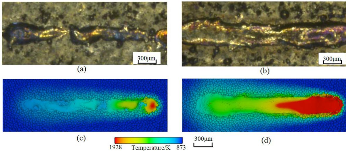
**Caption:** Experimental and simulation results of (a)(c) balling effect and (b)(d) single-track non-uniformity.
