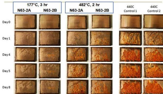
B117 Salt Fog Testing results show significantly improved corrosion resistance over 440C
