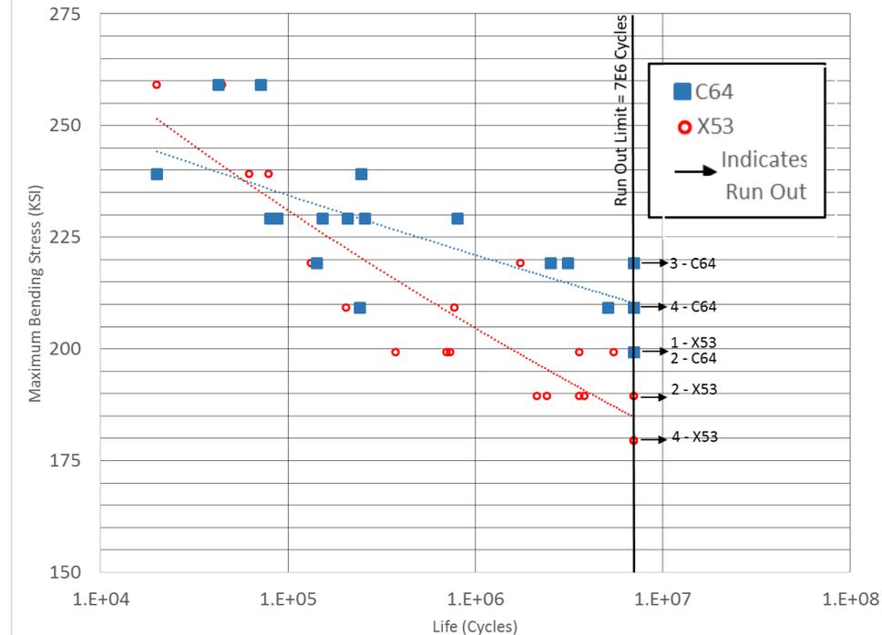
*Greater core strength of C61 steel leads to significant improvement in axial fatigue performance*
