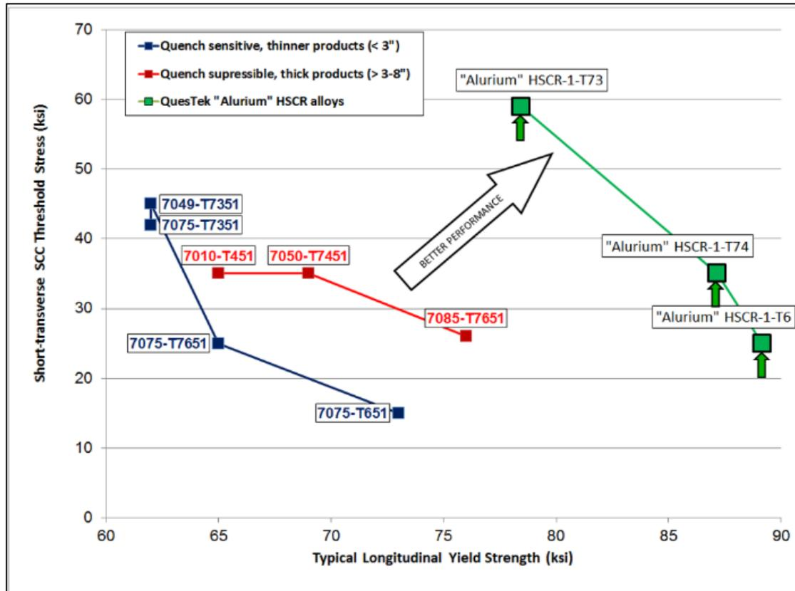
QuesTek "Alurium" alloys achieve a combination of strength and transverse SCC resistance significantly better than any incumbent aerospace aluminum alloy (including 7050-T74)
