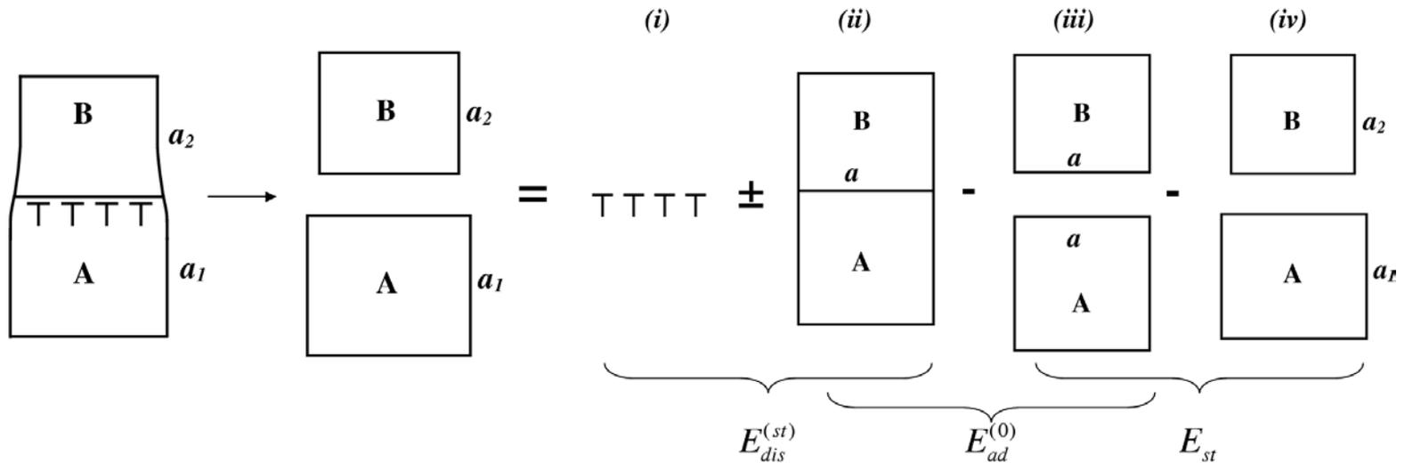
**Adhesion energy:**  $E_{ad} = E_{ad}^{(0)} - E_{dis}$ ;  $E_{ad}^{(0)}$  - ideal work of separation
